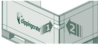
Once the load is introduced and secured within it, close the clipping crate box by placing the lid and clips corresponding to:
