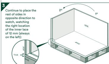
Always place the clips from the inside slot until it fits into the adjacent side slot:
